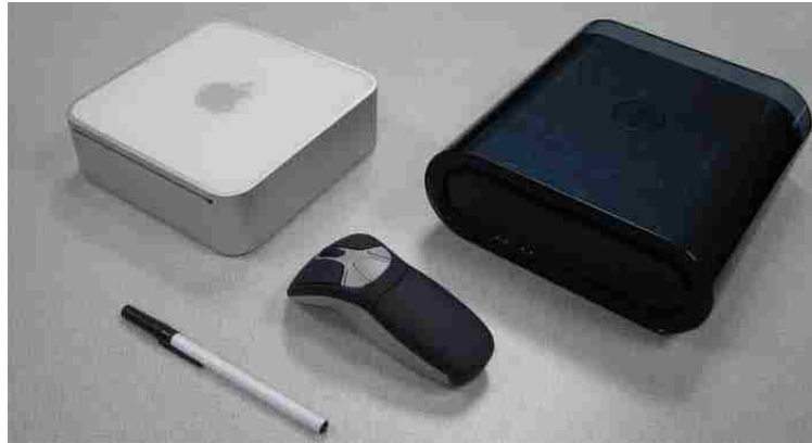
Figure 33: Small computers serving as set-top boxes. Left shows an Apple Mac Mini and right shows a Dell Studio Hybrid. Pen and remote are shown for size comparison.
